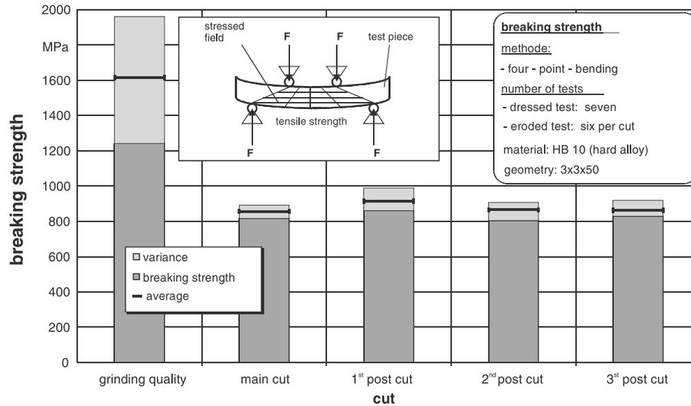
Fig. 3. Bending strength at use of a conventional technology strategy with the WEDM.
