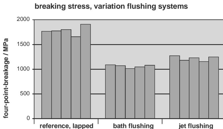
Fig. 7. Comparison of the bending fracture stress with variation of the flushing conditions in the main-cutting.
