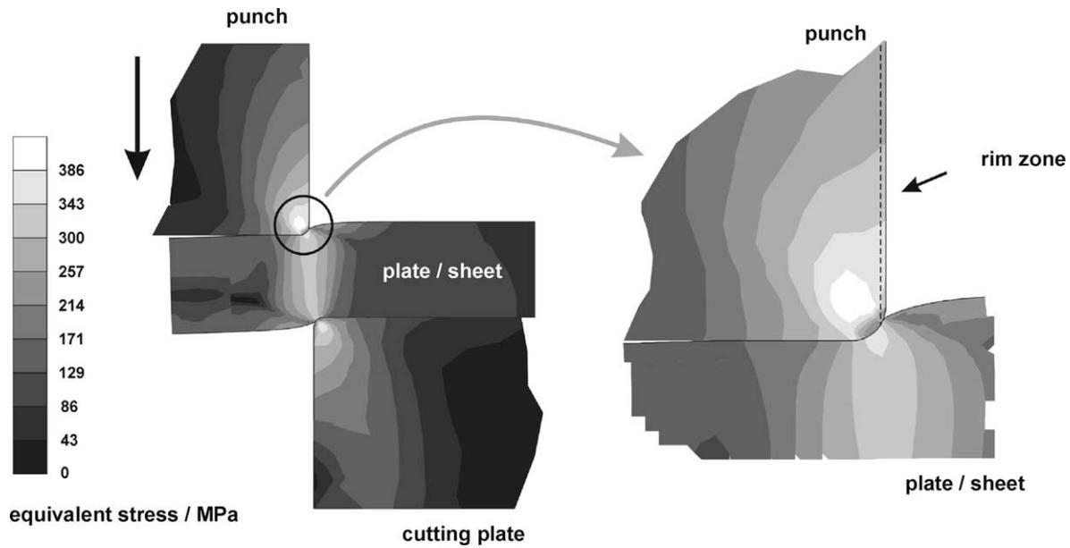
Fig. 1. Strain on the active instrument elements while the sheet cutting.
