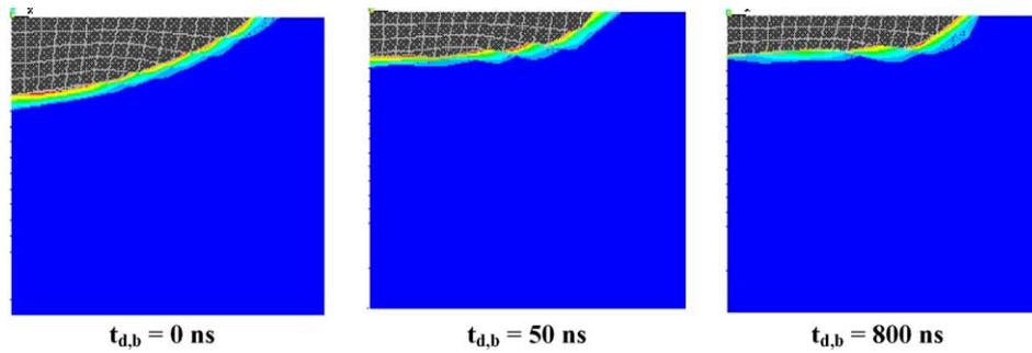
Fig. 5. Change of the thermal-affected zone by needle pulse time displacement.
