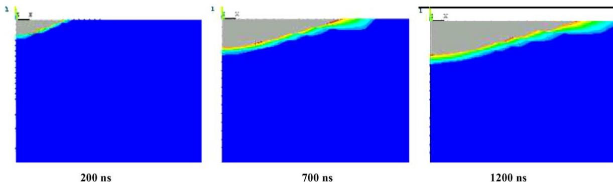
Fig. 4. Simulation of thermal influence of WEDM surfaces.
