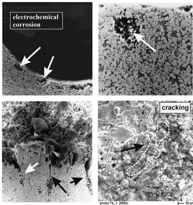
Fig. 2. Damages of the rim zone due to WEDM.
