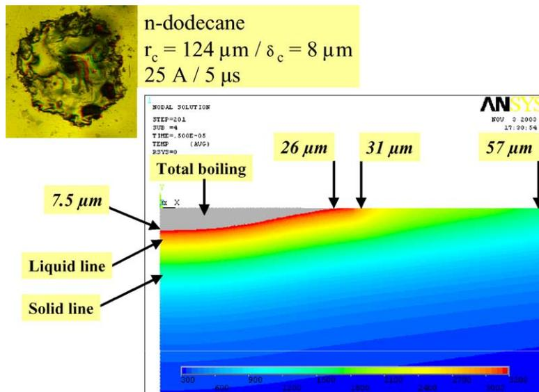
Fig. 8. Simulation of the thermal-affected zone and comparison with measured crater geometry (25 A, 5 μs).
