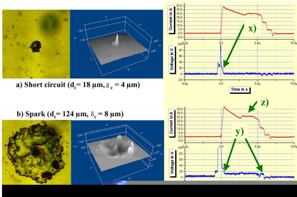
Fig. 4. Crater geometry of short circuit and spark discharge [6].
