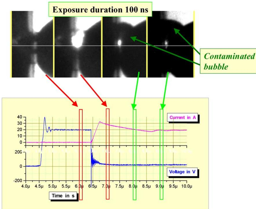
Fig. 3. Influence of the gas bubble of the emission effect of the plasma channel.
