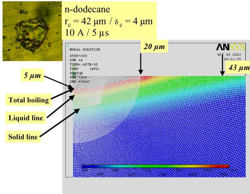
Fig. 7. Simulation of the thermal-affected zone and comparison with measured crater geometry (10 A, 5 μs).
